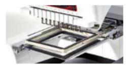
Double-sided Clamp Frame M (100 x 100 mm) One side with brush type (for general fabric).
